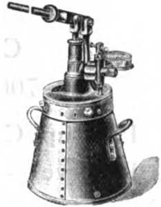
HYDR. TESTING PUMP.
